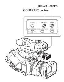
**CONTRAST:** For adjusting the brightness **BRIGHT:** For adjusting the brightness When you view the knob from the front, clockwise rotation increases the level and counterclockwise rotation decreases it.
